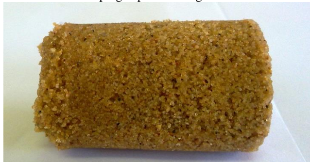
Fig-1, Sand Plug prepared in static condition
