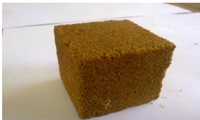
Fig-2, Sand Cube for compressive strength
