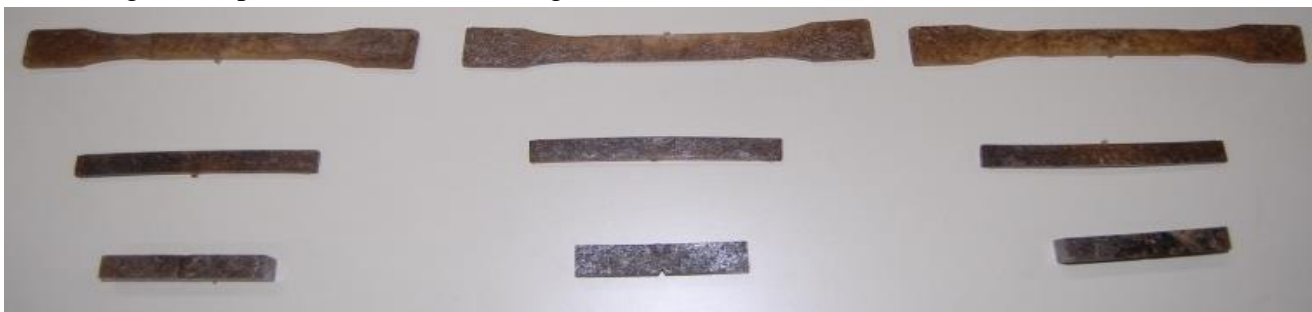
Figure 2: Specimens for Tensile, Bending and Impact test
