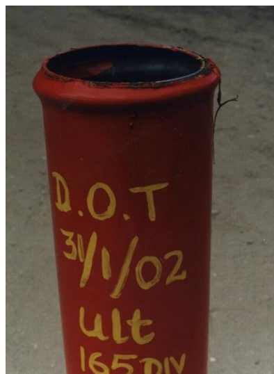
Figure 10. Bulging failure of hollow steel tubular column specimen
