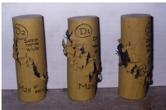
Figure 11 Failure pattern of CFST composite column specimens for L/D = 3
