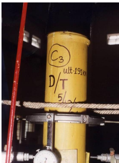
Figure 9. Local buckling and bulging failure at the ends of CFST steel only loaded column
