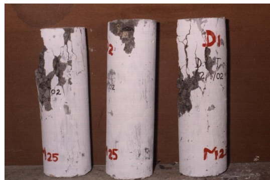
Figure 12 Failure pattern of RC column specimen for L/D = 3
