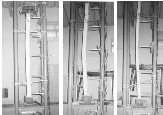
Fig.3 Buckling of columns
