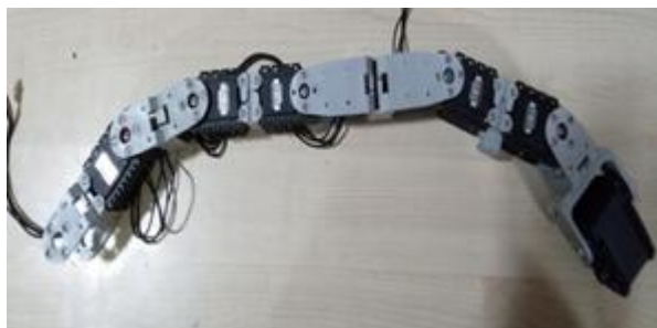
Figure 5: Assembled hardware Robotic arm by proposed method
